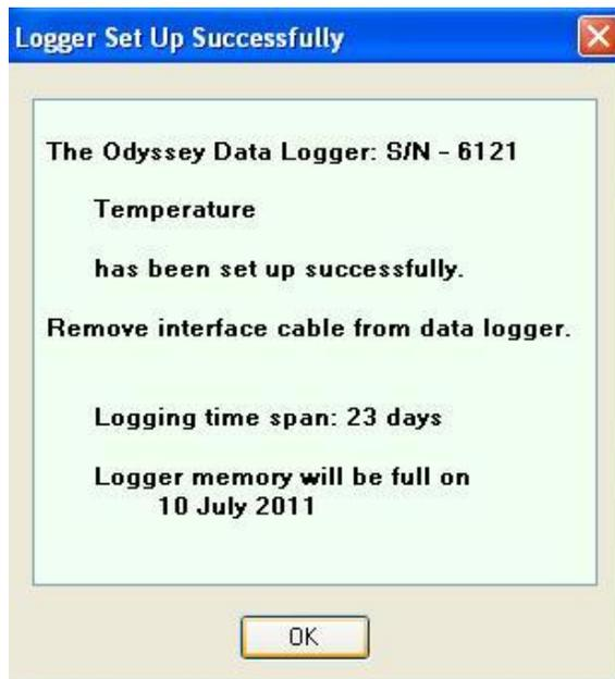
**Note: All Odyssey Data Loggers are equipped with non-volatile memory, so data will be preserved even in the case of battery failure.**
