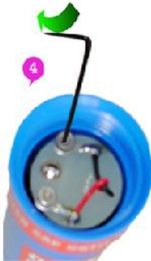
Replacement battery assemblies include the front fibreglass disk soldered to the batteries. These will be available from Dataflow Systems.
