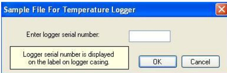
User must enter the logger serial number to create a site file using Sample Site File option.
